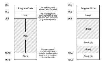
Figure 26.1: Single-Threaded And Multi-Threaded Address Spaces
